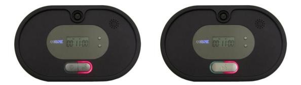
The portable microphone units are microcomputer controlled conference units with loudspeaker, which is automatically switched off when the microphone is activated. Connected with KLOTZ gooseneck microphone, it's completely conference unit. The units have 2 m cable for daisy chain connection.
