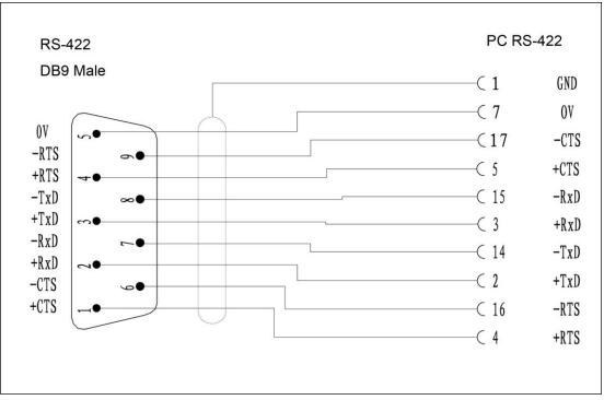
Cable between PC and RS-422 must be less than 1000m.
