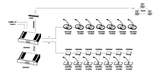
This is an application with 2 microphone bus and expands 2 central controllers. With video tracing system, the camera will connect to the speaker.
