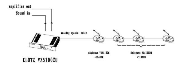
This is an application of signal chain. And the microphone volume controlled by the central controller.
