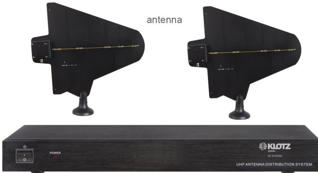
Antenna amplifier consists of an antenna distributor and two directional antenna, can be accessed by multiple conference controller, so that the received signal to obtain better signal noise ratio, to extend the receiving distance and enhance system stability, providing four sets of power output to the conference controller, easy to install.
