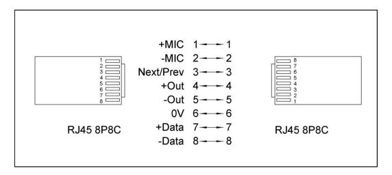
Cable between two VZ 5600CU must be less than 250m.
