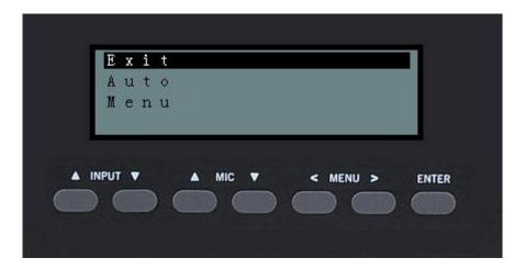
Pressing the MENU </> for option and ENTER to determine the function.
