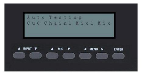
Manual testing: System would turn on the first microphone on the BUS 1 after starting the manual testing, press '< or >' buttons below MENU to open the previous or next microphone. The status display of opening microphones on the central controller would be the same as it is for automatic testing.
