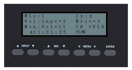
Mic: 1 1 connected microphone unit in the system
