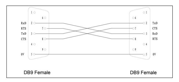
Cable between 2 DB9 female connectors must be less than 10m.
