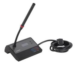
The portable microphone units are microcomputer controlled conference units, contained KLOTZ gooseneck microphone, it's completely conference unit.
